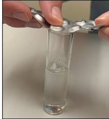
Placing Tablet into Test Tube
