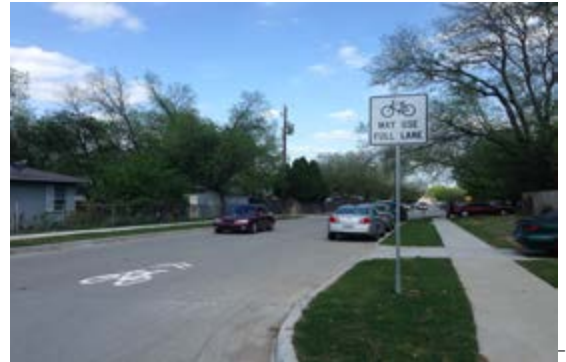
"Sharrows" and signage, like these on E. Lovers Lane, remind bicyclists and motorists to share the road space with each other
